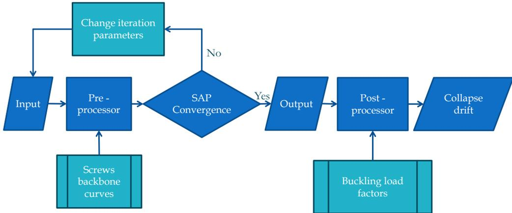
**Figure 4.1 - Schematic flow chart of the automatic tool for seismic assessment of plasterboard partition**
