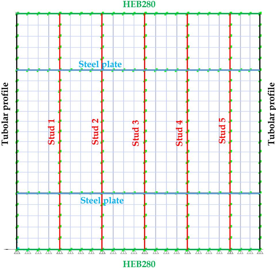
Figure A. 9 - Fem model in Sap2000 of the partition P-3
