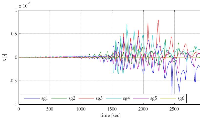
**Figure 2.23 - Strain gauges recordings on the steel studs of partition P-3 during the test**
