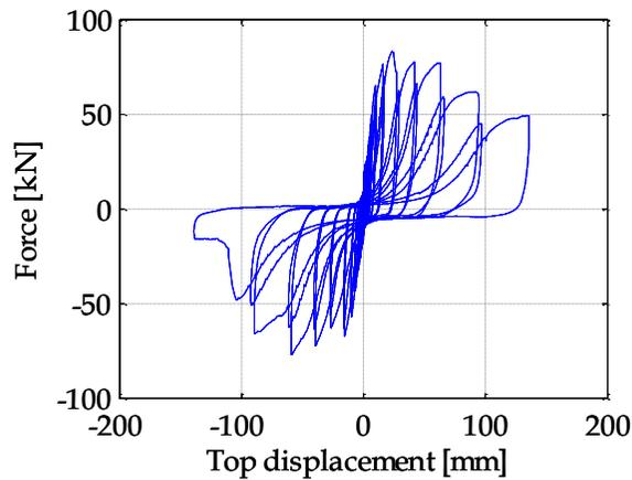
**Figure 2.13 - Hysteretic curve exhibited by the partition P-1 under the selected test protocol**
