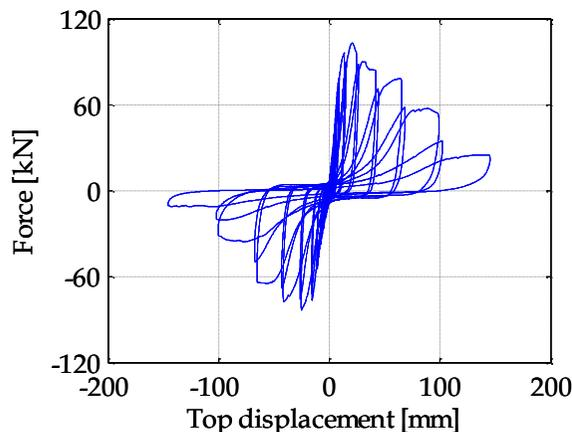
Figure 2.21 - Hysteretic curve exhibited by the partition P-3 under the selected test protocol
