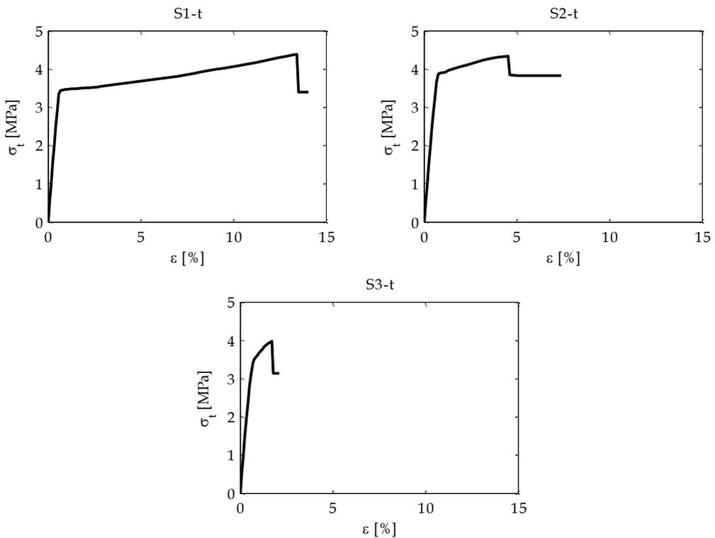
Figure 5.11 - Stress-strain curves for cubic specimen subject to tensile tests
