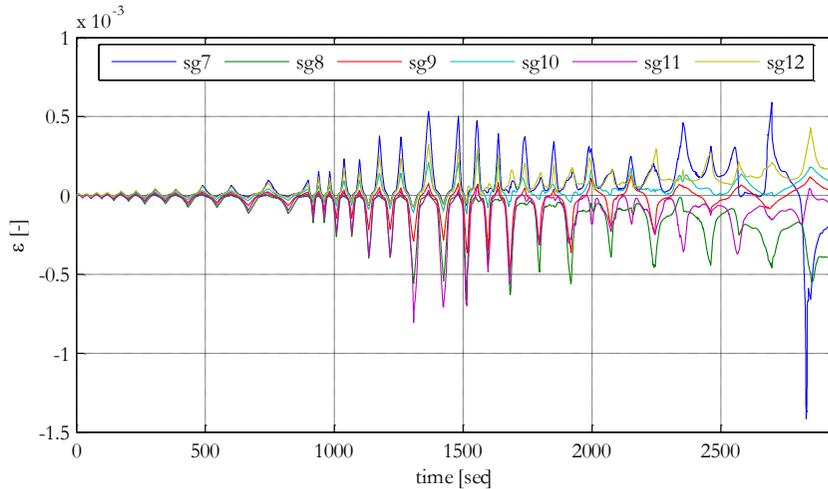
Figure 2.24 - Strain gauges recordings on the plasterboard of partition P-3 during the test
