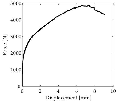
**Figure 3.13 - Force - displacement curve of panel-to-stud connection for BA18S plasterboard panel**
