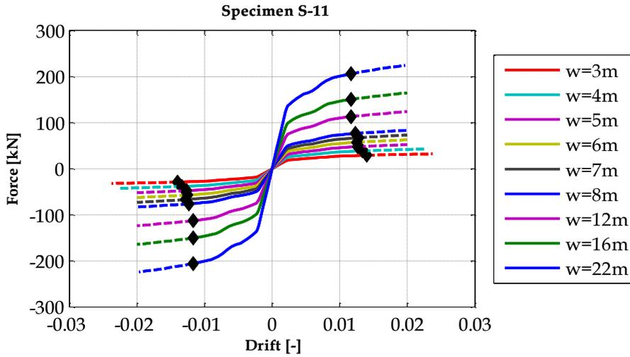
Figure 4.47 - Force vs drift pushover curve for S-11 partition at different widths
