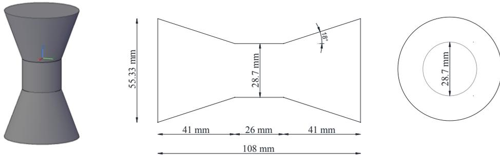
**Figure 5.3 – Configuration of the specimen for tensile test**
