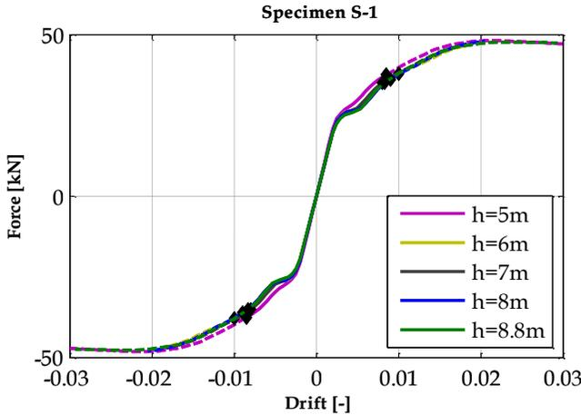
Figure 4.15 - Force vs drift pushover curve for S-1 partition at different heights
