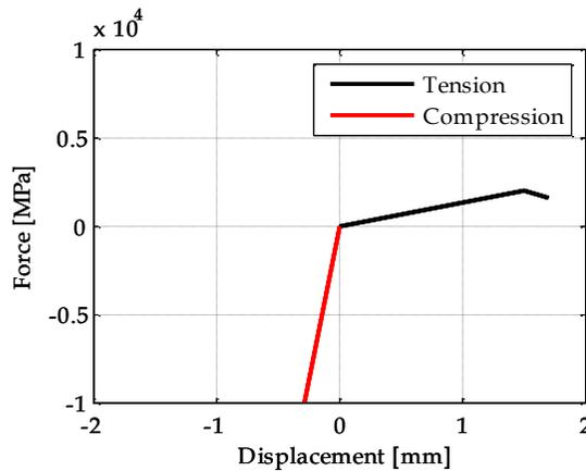
Figure 3.49 - Force-displacement curve for contact element
