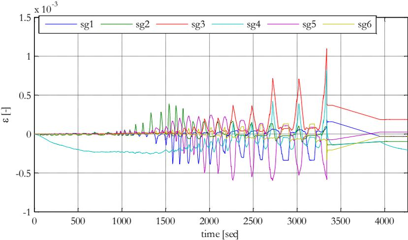
Figure 2.26 – Strain gauges recordings on the steel studs of partition P-4 during the test
