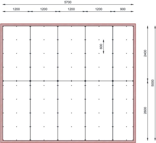
Figure 2.4 - Typical panel arrangement in the internal layer
