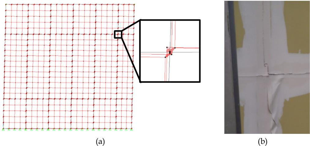
**Figure 3.28. (a) Deformed shape of the analytical model and (b) particular of the board overlap in the corner.**
