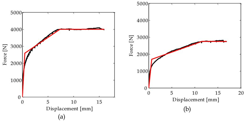
**Figure 3.20 - Trilinear envelope of the backbone curve for BA13 screwed connection in (a) configuration 1 and (b) configuration 2**
