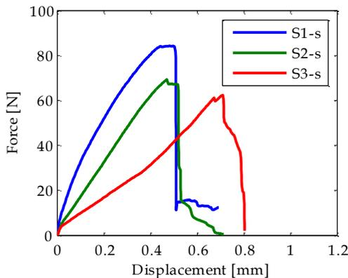
Figure 5.13 - Force vs displacement in for hybrid foam subject to shear test
