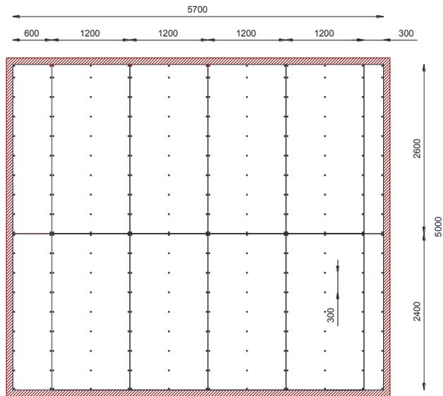
Figure 2.5 - Typical panel arrangement in the external layer
