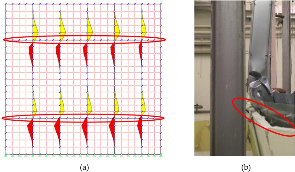
**Figure 3.27. (a) Bending moment diagram on studs of P-3 specimen at the last step analysis crossing horizontal joints (in red circles) and (b) observed damage on stud below the horizontal joint (red circled).**
