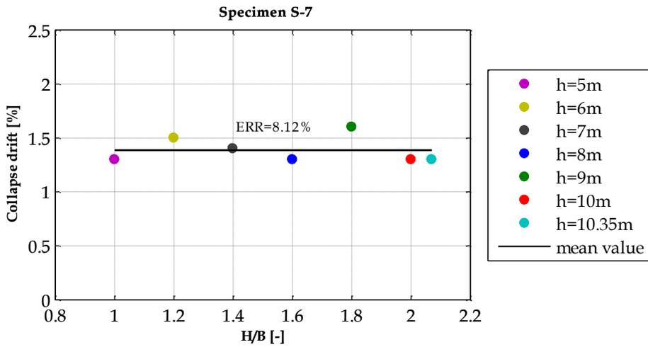
Figure 4.27 - Collapse drift vs H/B ratio for partition S-7
