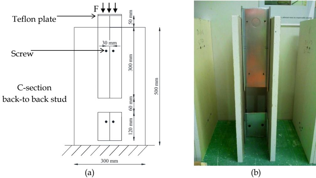
Figure 3.10 - (a) Schematic view of the tested specimen dimensions (in mm) and (b) assembled specimen before testing.
