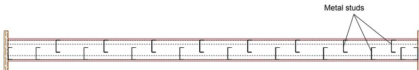
Figure 2.6 - Plane view of the tested partitions with double layer of staggered steel stud
