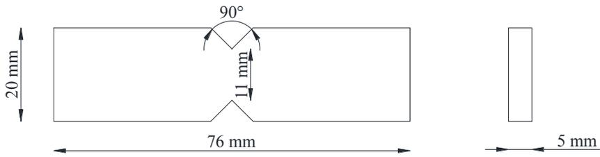
**Figure 5.5 - Specimen configuration for shear tests**
