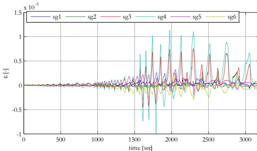
Figure 2.18 – Strain gauges recordings on the steel studs of partition P-2 during the test
