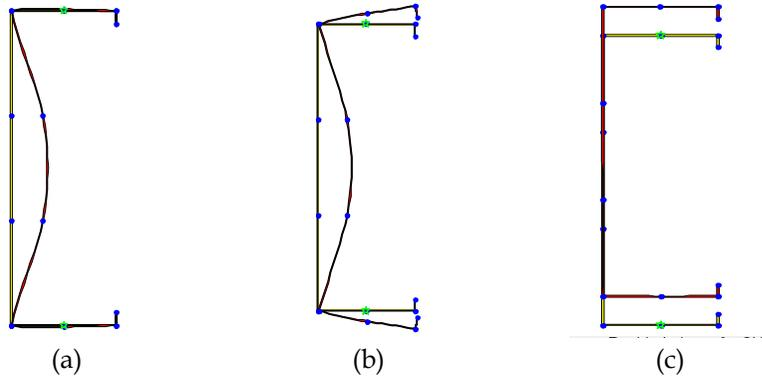
**Figure 3.29. Three different buckling failure modes: (a) local buckling, (b) distortional buckling and (c) global buckling.**
