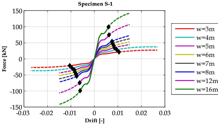
Figure 4.35 - Force vs drift pushover curve for S-1 partition at different widths
