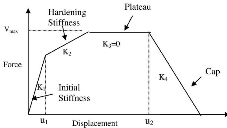
Figure 3.4 - Backbone curve of spring model for plasterboard partition (after Kanvinde and Deierlein, 2006)
