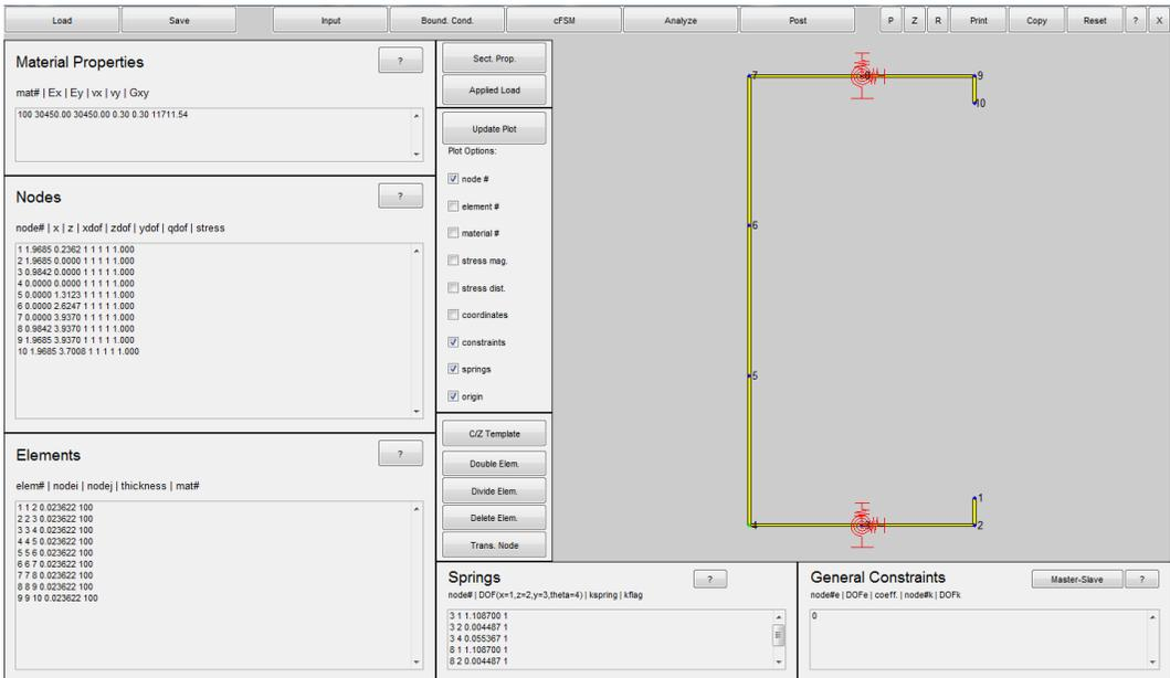
Figure 3.34 – Main screen of CUFEM software for input data of covered stud
