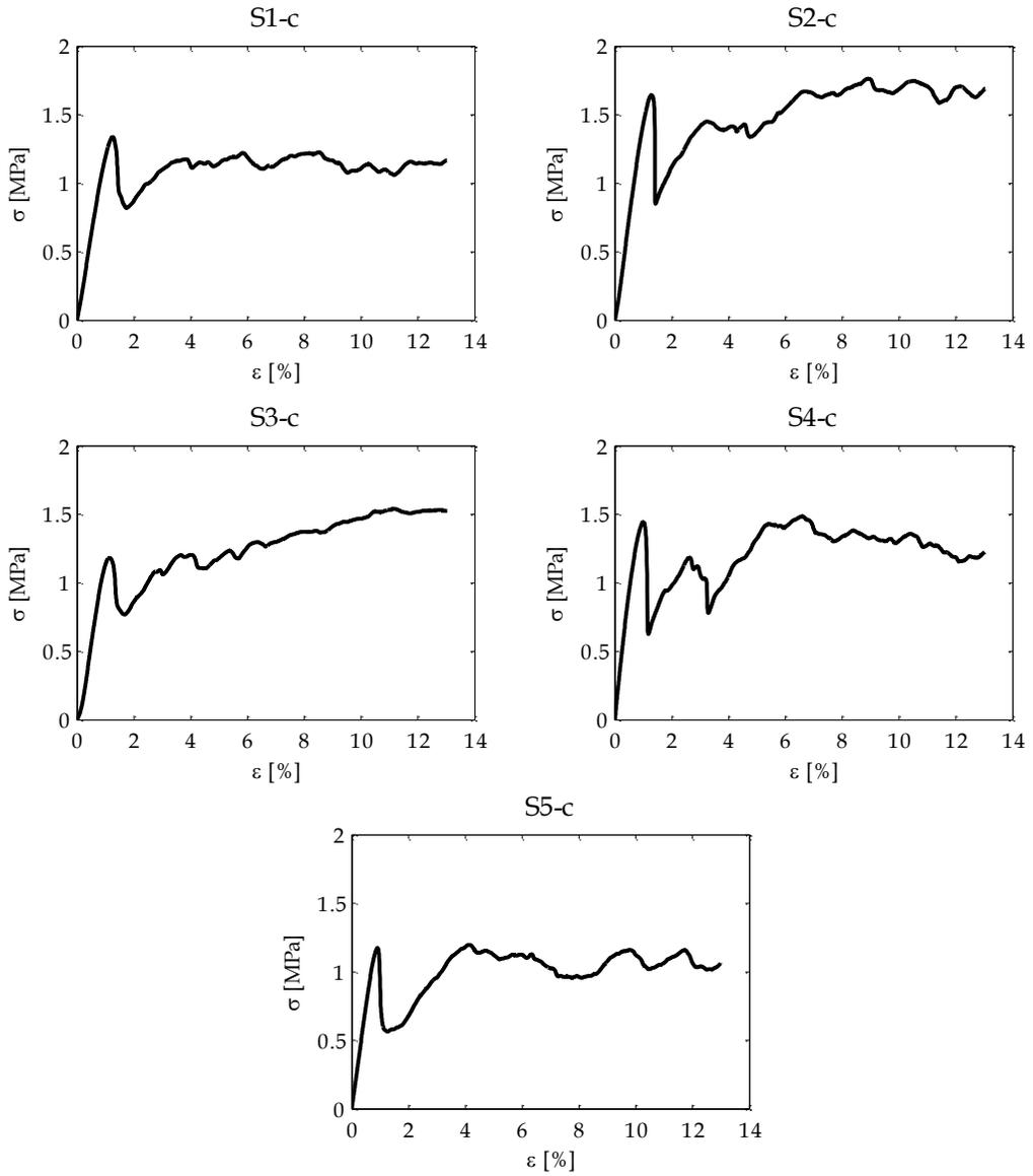
Figure 5.8 - Stress-strain curves for cubic specimen subject to compression tests
