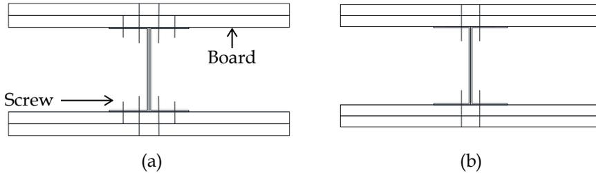
**Figure 3.12 - (a) Configuration 1 of the panel-to-stud connection providing 4 screws for each side of the partition and (b) configuration 2 providing two screw for each partition side**
