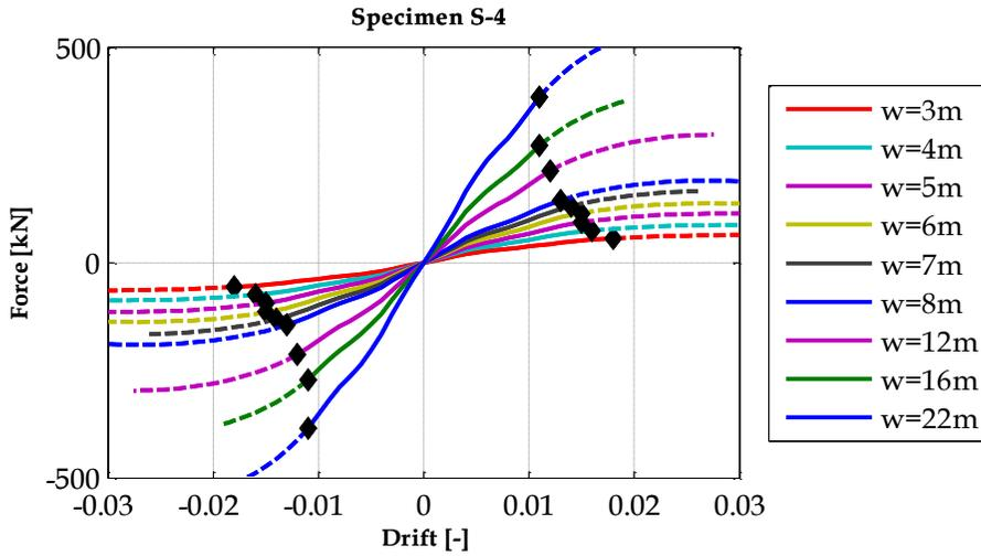
Figure 4.39 - Force vs drift pushover curve for S-4 partition at different widths
