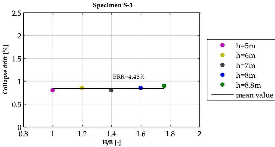
Figure 4.19 - Collapse drift vs H/B ratio for partition S-3
