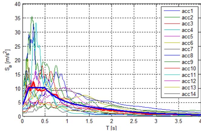
**Figure 2.8 – Spectra of the records considered in the input definition study and EC8 spectrum**
