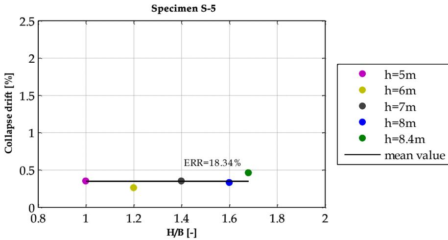
Figure 4.23 - Collapse drift vs H/B ratio for partition S-5
