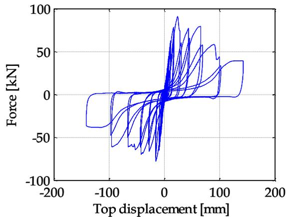
Figure 2.17 - Hysteretic curve exhibited by the partition P-2 under the selected test protocol
