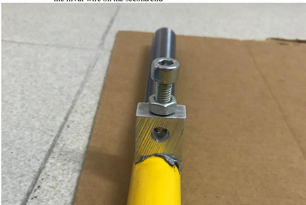
d) Photograph of aluminium elements produced to fix the invar wire on the first end
