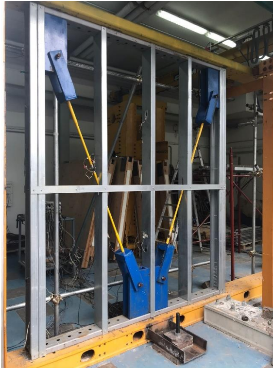
Figure 4-14 M Configuration wall tested
