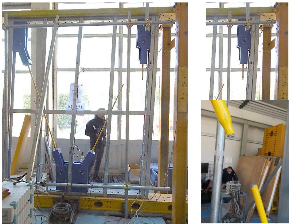
Figure 4-24 M_M1 test: collapse mechanism
