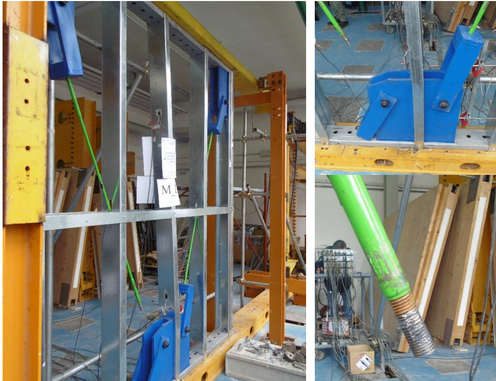
Figure 4-22 M_L1 test: collapse mechanism
