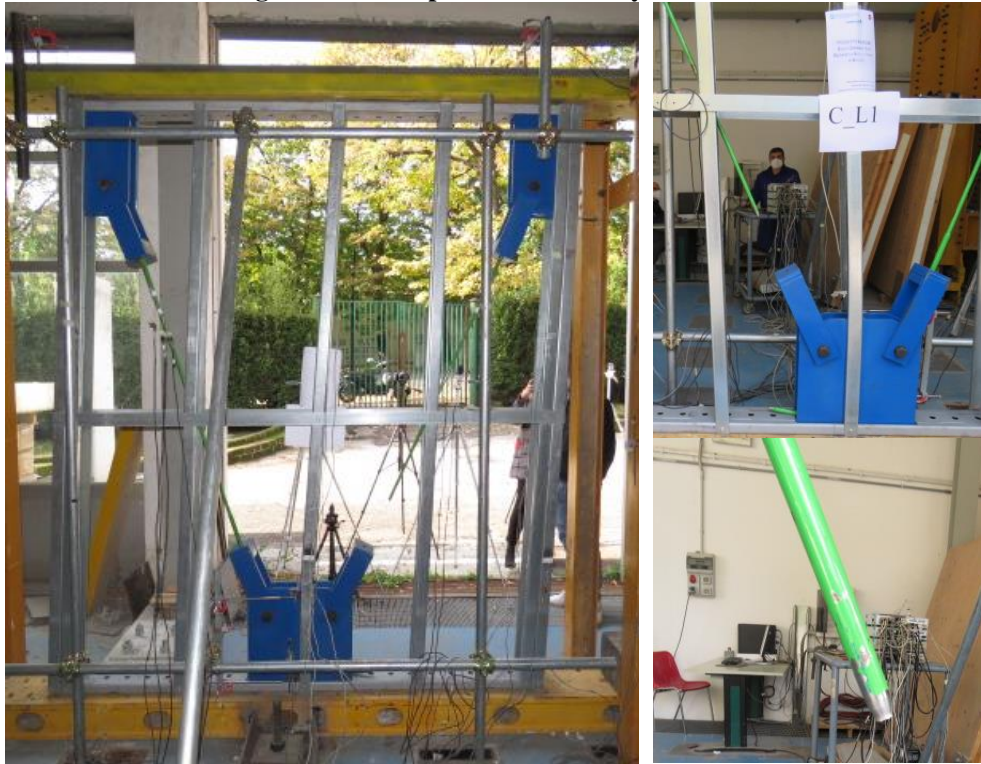
Figure 4-30 C_L1 test: collapse mechanism
