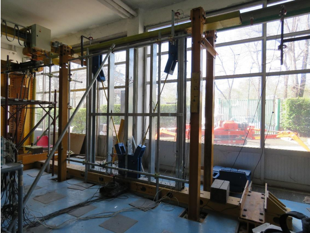
Figure 4-16 Wall test set-up
