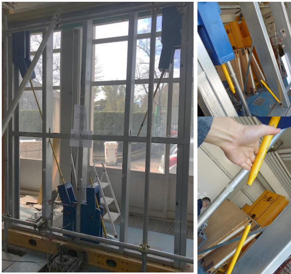
Figure 4-31 C_M1 test: collapse mechanism
