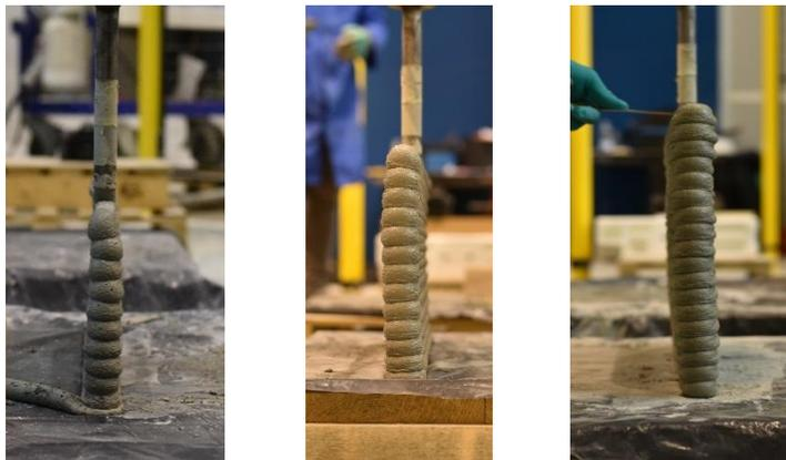
*Figure 2-45: Printed specimens just before the failure.*
