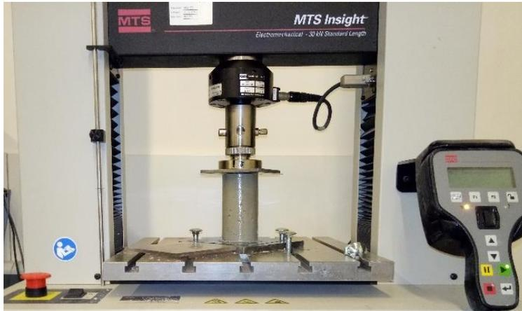
Figure 2-19: Testing setup: MTS electromechanical Universal Testing Machine.
