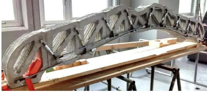
Figure 1-7: External reinforcement system with tightened bars [32]
