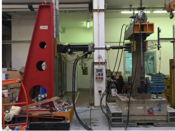
**Figure 4.3.** Experimental setup for the cyclic pushover tests.
