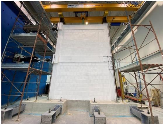
**Figure 3.5.** Front view of one full-scale RC frame with the pseudo-dynamic test setup.
