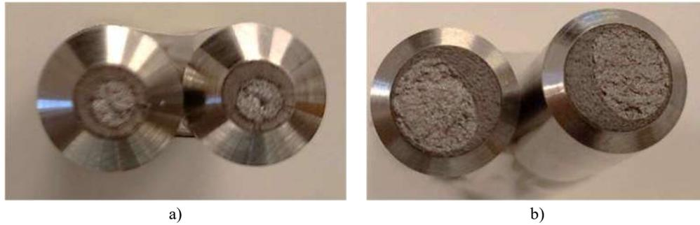
**Figure 4.4** Macroscopic fracture surfaces for statically tested specimens: a) T5001 and b) T7501.
