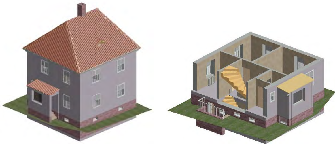
Figure 3.26: As-built BIM model of the building (left) and axonometric split (right)
