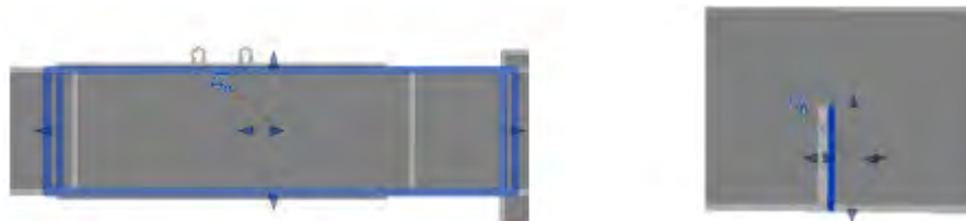
Figure 4.2: Modelling the passing (left) and not-passing (right) cracks in a BIM environment.
