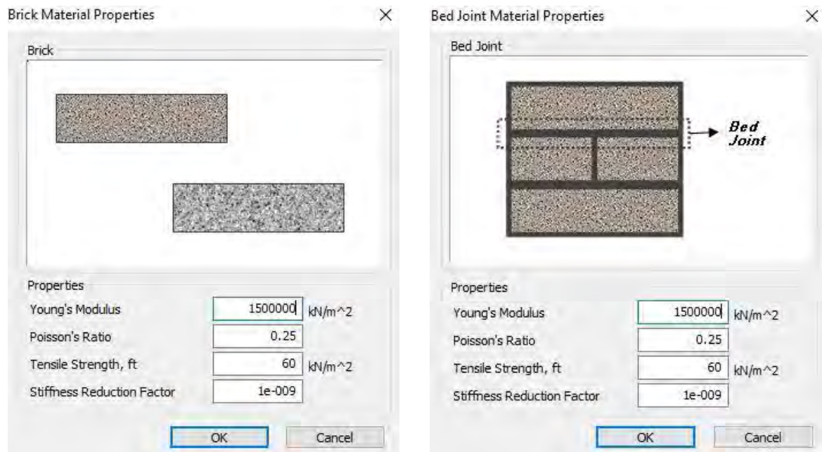
Figure 3.32: Mechanical parameters of masonry material according to Strumas Model.
