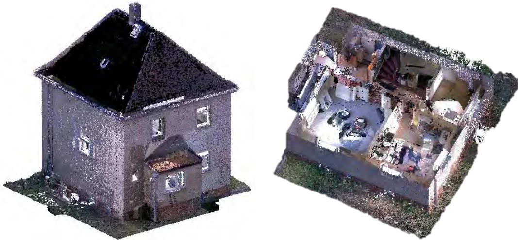
Figure 3.22: Point cloud obtained with a laser scanner survey (left) and axonometric split (right)
