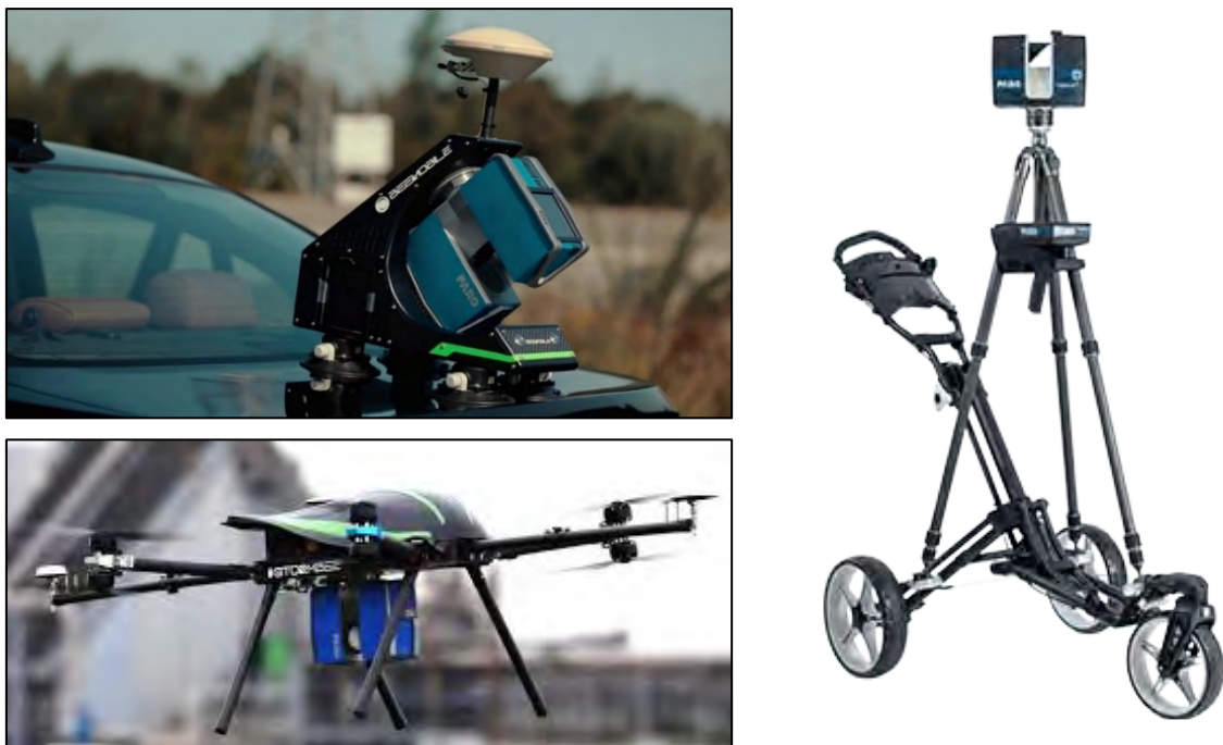
Figure 3.7: Stormbee, Beemobile and FARO Swift systems to upgrade static laser scanners in dynamic ones
