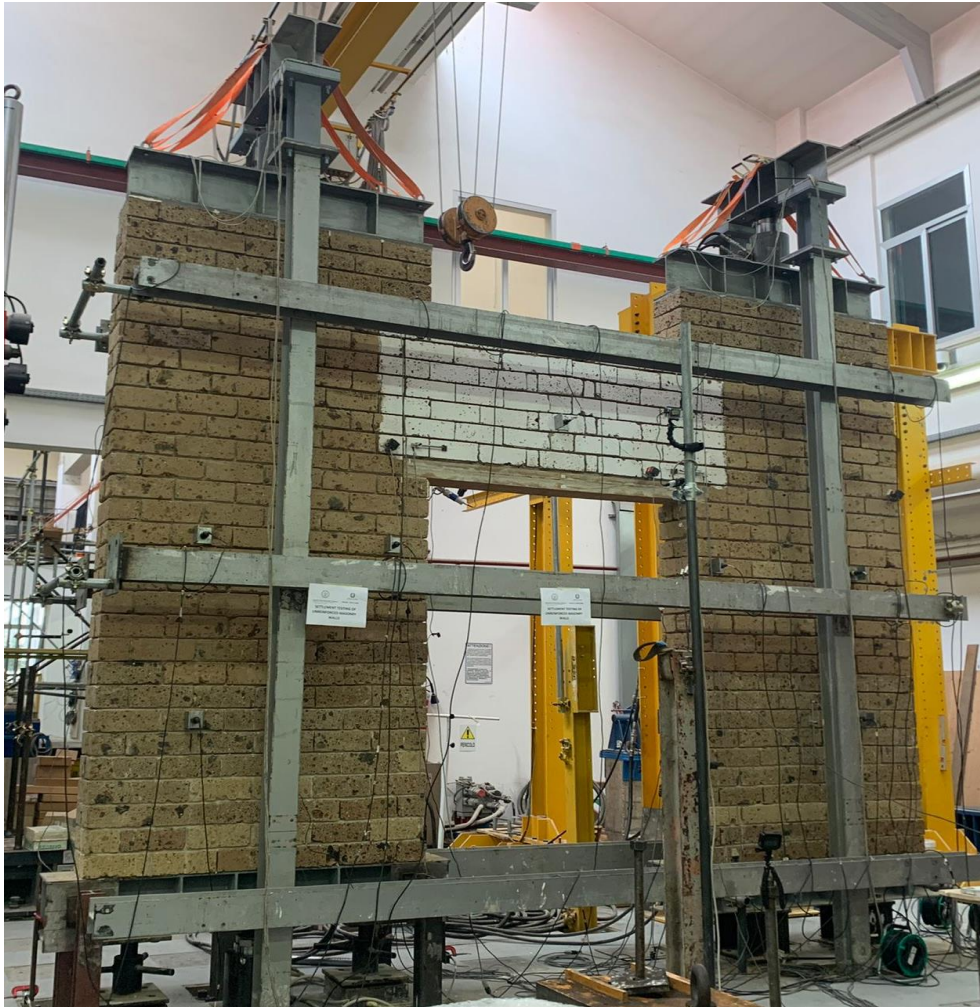
Figure 42. Experimental setup of deteriorated URM under settlement load
