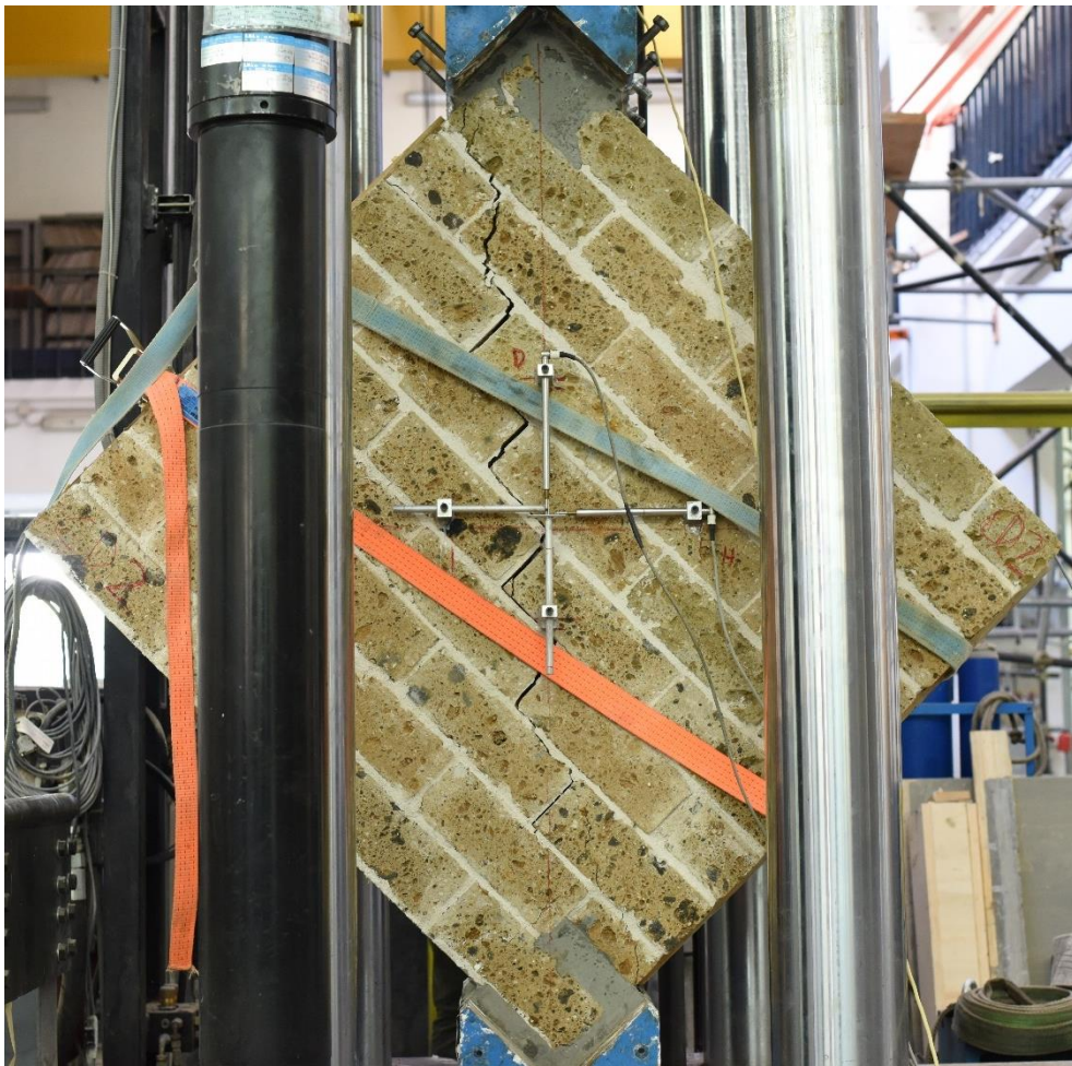
Figure 27. Crack pattern of specimen TM_D_2
