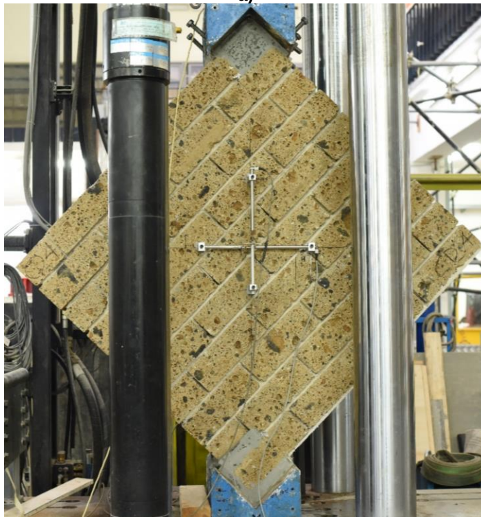
Figure 23. Experimental setups of specimens subjected to diagonal compression in configuration (a) intact and (b) deteriorated.
