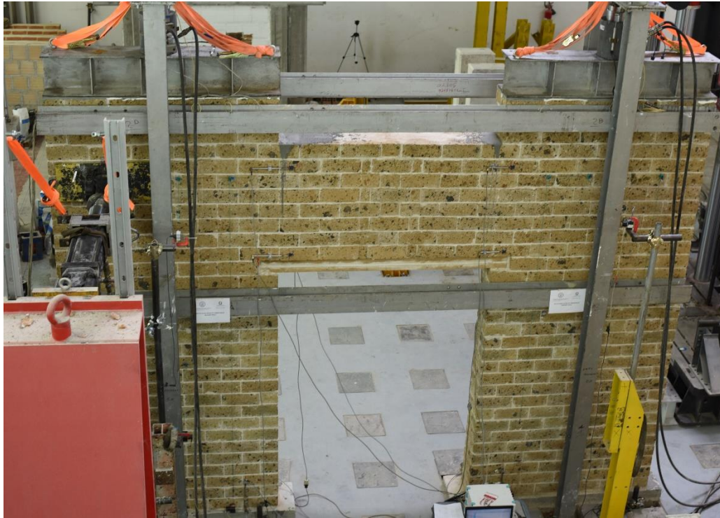
Figure 52. Experimental setup of intact URM under out-plane load, frontal side
