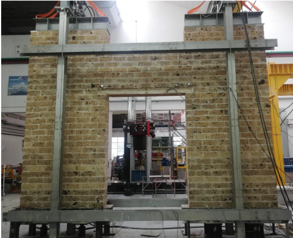
Figure 41. Experimental setup of intact URM under settlement load
