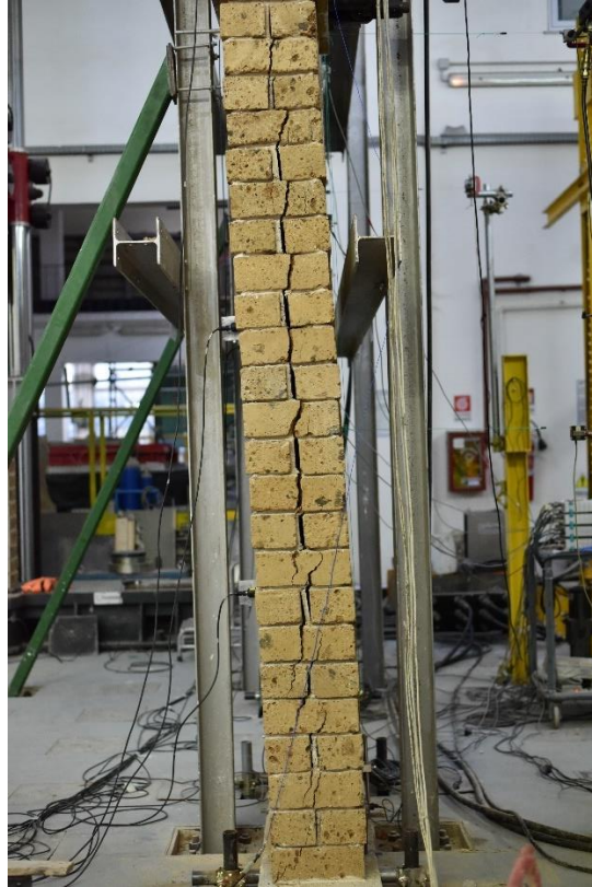
Figure 64. Crack pattern ,deteriorated URM, lateral view
