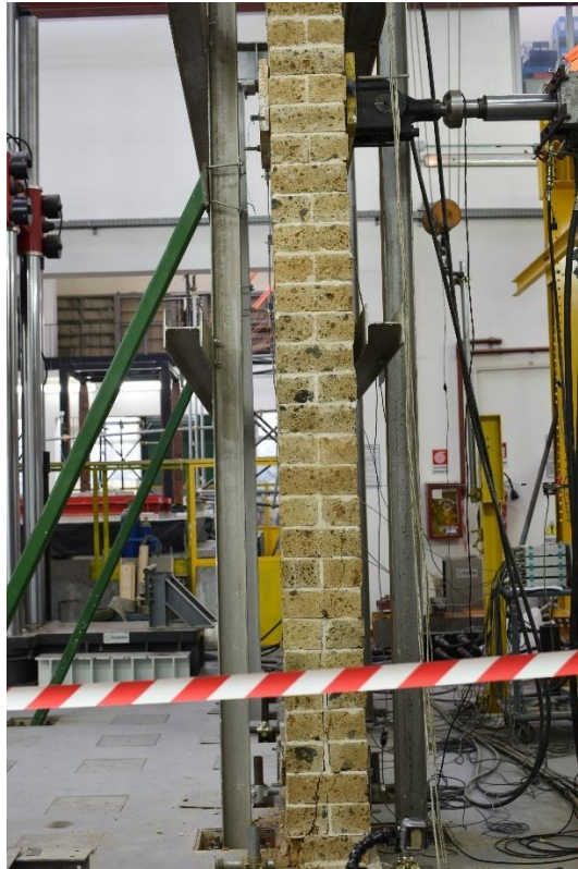
Figure 59. Crack pattern, intact URM, lateral view
