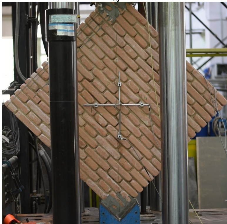
Figure 6. Experimental setups of specimens subjected to diagonal compression in configuration (a) intact and (b) deteriorated.
