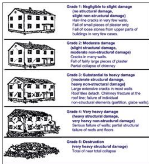
Figure 93. EMS'98 scale damage levels (Grünthal, 1998) for masonry buildings.
