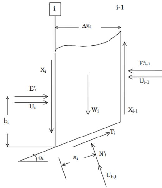
Figure A-6. Forces acting on a slice through a sliding mass defined by a slip surface.
