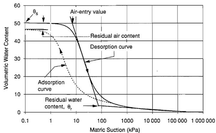
Figure 2-6. Typical soil-water characteristic curve (Fredlund and Xing 1994).
