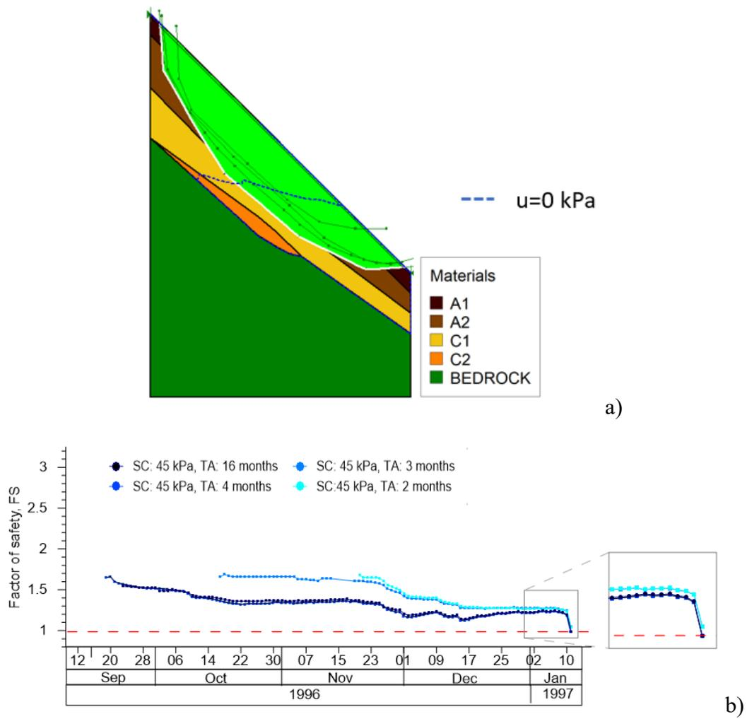
Figure 6-7. Slope stability analyses for the Pozzano section: a) slip surface on 10<sup>th</sup> January 1997; b) Minimum safety factor, FS, over time: results of analyses of group A of duration 16, 4, 3 and 2 months.
