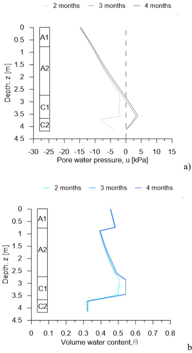
Figure 6-9. Results along the vertical profile of the Pozzano section on 10<sup>th</sup> January 1980: a) distribution of pore water pressure; b) distribution of volumetric water content.
