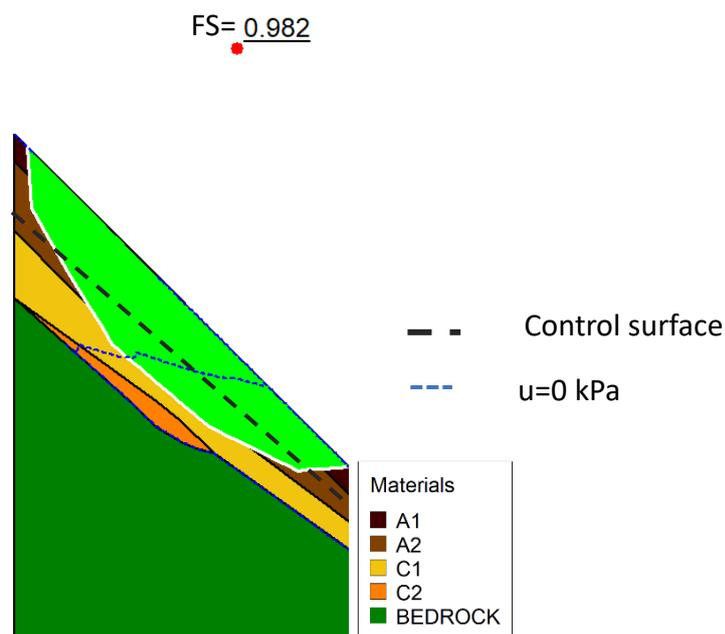
Figure 7-1. Slope stability analyses for the Pozzano section: sliding surface occurring on 10<sup>th</sup> January 1997.
