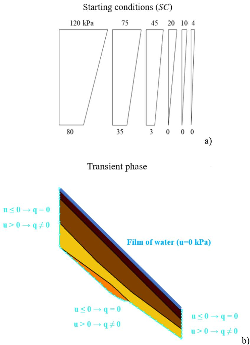
Figure 5-2. Analyses of E group on Pozzano section: a) suction profiles at starting condition; b) boundary conditions at transient phase
