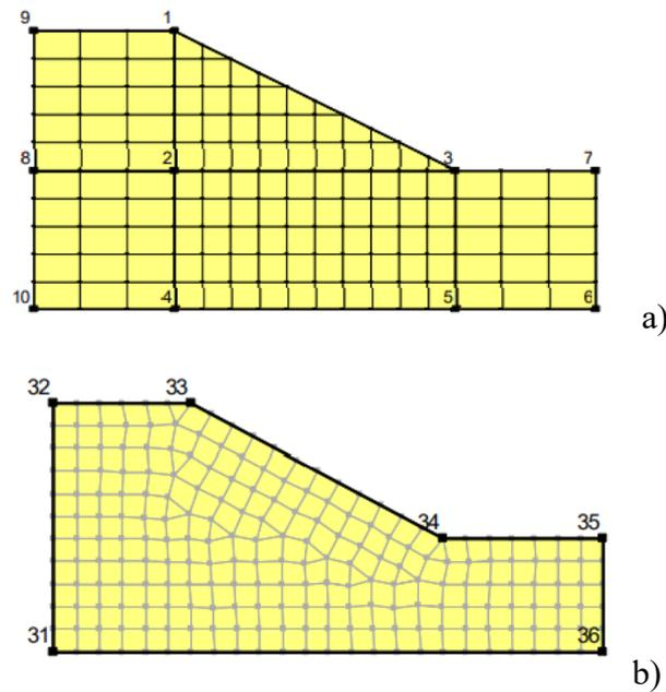
Figure A-4. SEEP/W: a) structured mesh; b) mixed quad and triangle unstructured mesh (Seepage modelling with SEEP/W, 2012).
