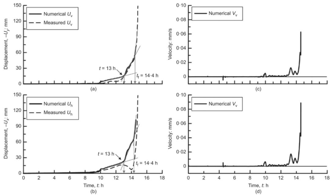
Figure 2-35. Field data and results of analyses: Evolution of (a), (b) displacements and (c), (d) velocity at the slope surface at cluster 3 (Sitarenios et al. 2021)
