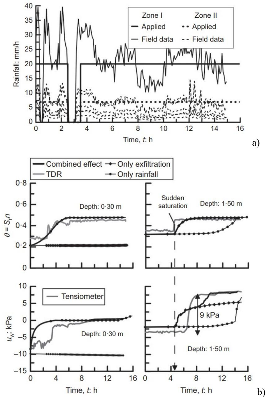
Figure 2-34. Field data and results of analyses: a) field rainfall data; b) Evolution of volumetric water content (above) and pore water pressure (below) at cluster 3. In (a) at a depth of 0.30 m and (b) at a depth of 1.5 m; for only exfiltration, only rainfall and for their combined effect (modified from Sitarenios et al. 2021)
