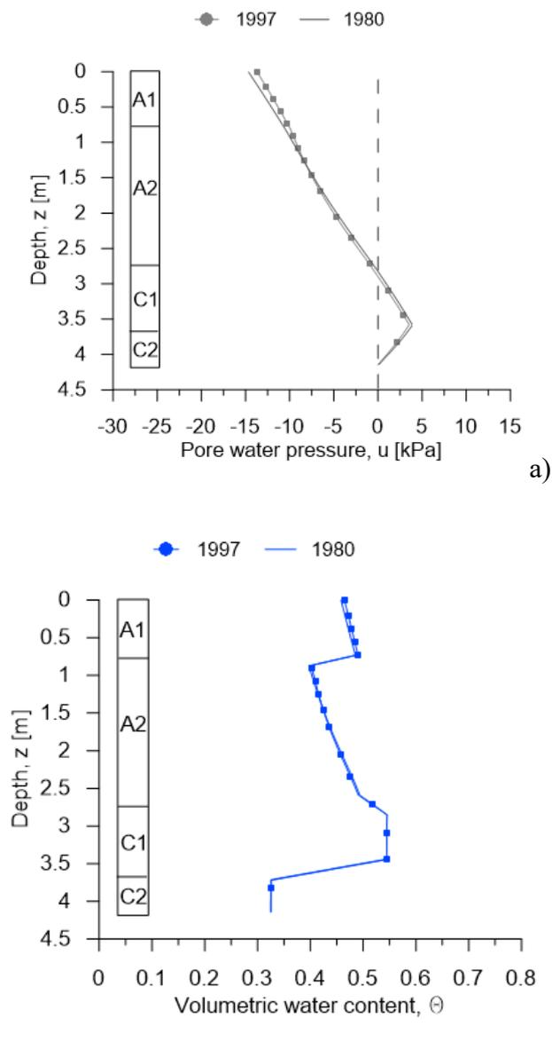
Figure 6-11. Results along the vertical profile of the Pozzano section on 25<sup>th</sup> December 1996 and on 10<sup>th</sup> January 1980 when the water storage, in both cases, have reached PWS value: a) distribution of pore water pressure; b) volumetric water content.
