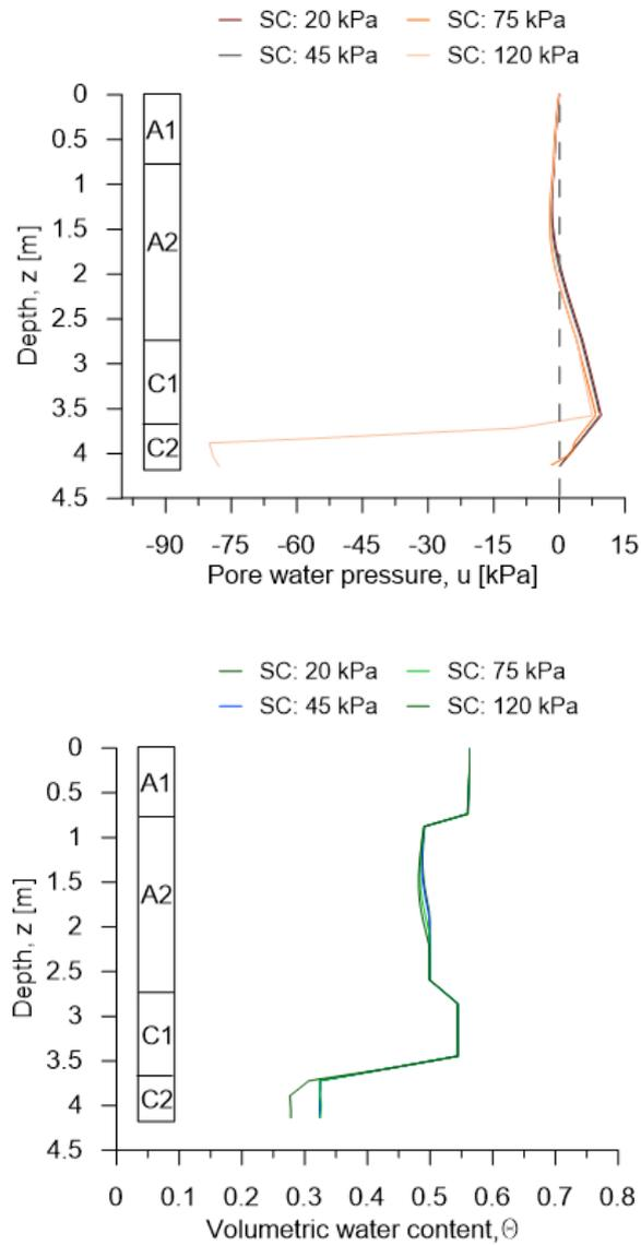
Figure 6-18. Results of analyses of C group along the vertical profile of the Pozzano section on 10<sup>th</sup> January 1997 (day of landslide): a) distribution of pore water pressure; b) volumetric water content.
