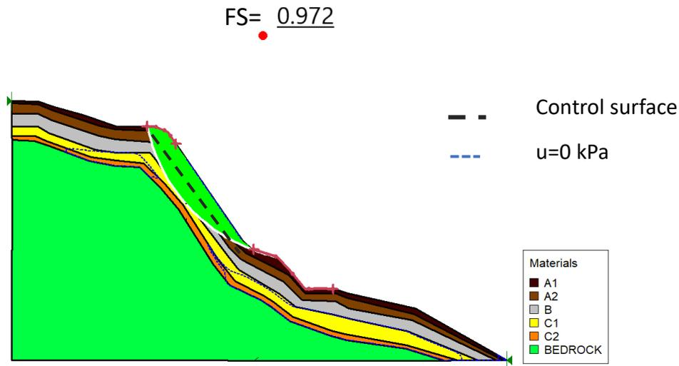
Figure 7-4. Slope stability analyses for the Pimonte section: sliding surface occurring on 10<sup>th</sup> January 1997.
