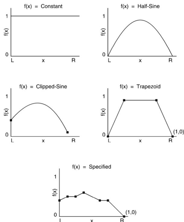
Figure A-7. Example of interslice force functions (stability modelling with SLOPE/W, 2012).
