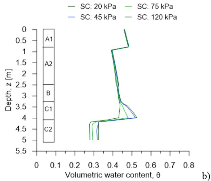
Figure 6-25. Results of analyses of D group along the vertical profile of the Pimonte section on 3<sup>rd</sup> January 1997 (7 days before the critical event): a) distribution of pore water pressure; b) volumetric water content.
