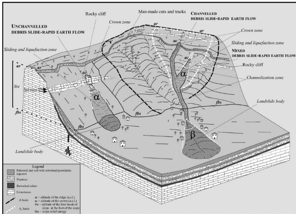
Figure 2-24. Scheme of the main morphology associated to debris flow type of landslide (Di Crescenzo and Santo, 2005).
