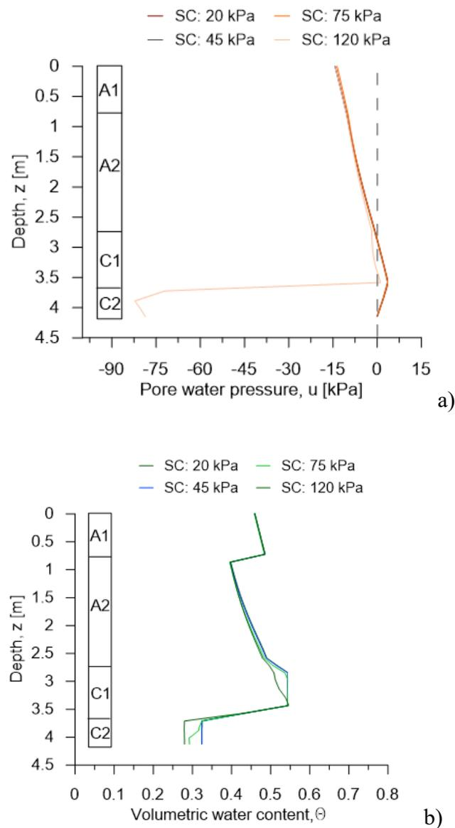
Figure 6-20. Results of analyses of C group along the vertical profile of the Pozzano section on 27<sup>th</sup> December 1996 (14 days before the landslide): a) distribution of pore water pressure; b) volumetric water content.
