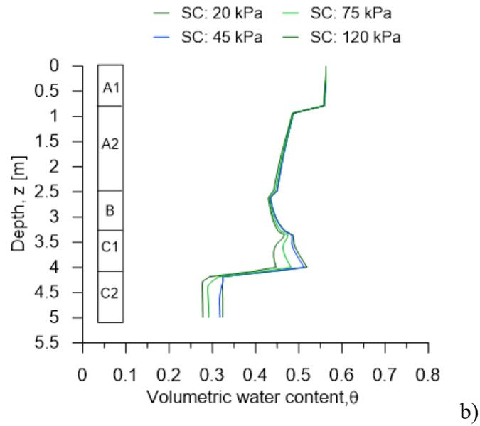
Figure 6-24. Results of analyses of D group along the vertical profile of the Pimonte section on 10<sup>th</sup> January 19967(days of the landslide): a) distribution of pore water pressure; b) volumetric water content.
