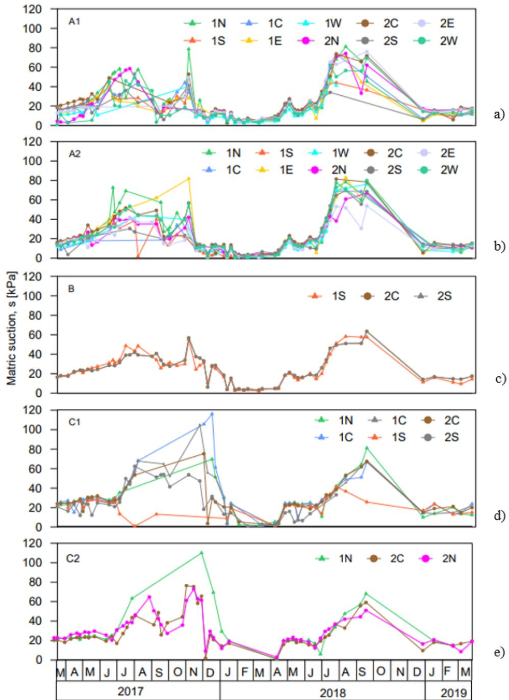
Figure 3-20. Matric suction monitored in cell 1 and cell 2 from 11 March 2017 to 26 March 2019 in: a) A1 soil layer; b) A2 soil layer; c) B soil layer; d) C1 soil layer; e) C2 soil layer.
