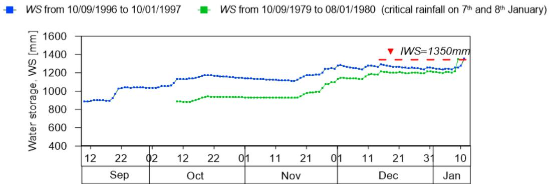
Figure 6-16. Pozzano section: volume of water stored, *WS*, from 10<sup>th</sup> September 1996 to 10<sup>th</sup> January 1997 and from 10<sup>th</sup> October 1979 to 8<sup>th</sup> January 1980 when the critical rainfall of 25 mm and 150 mm was applied.
