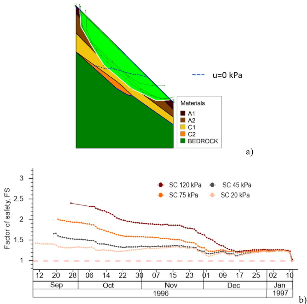
Figure 6-21. Slope stability analyses of C group for the Pozzano section: a) sliding surface relative to the triggering of landslides due to the event occurring on 10<sup>th</sup> January 1997; b) minimum safety factor,  $FS$ .
