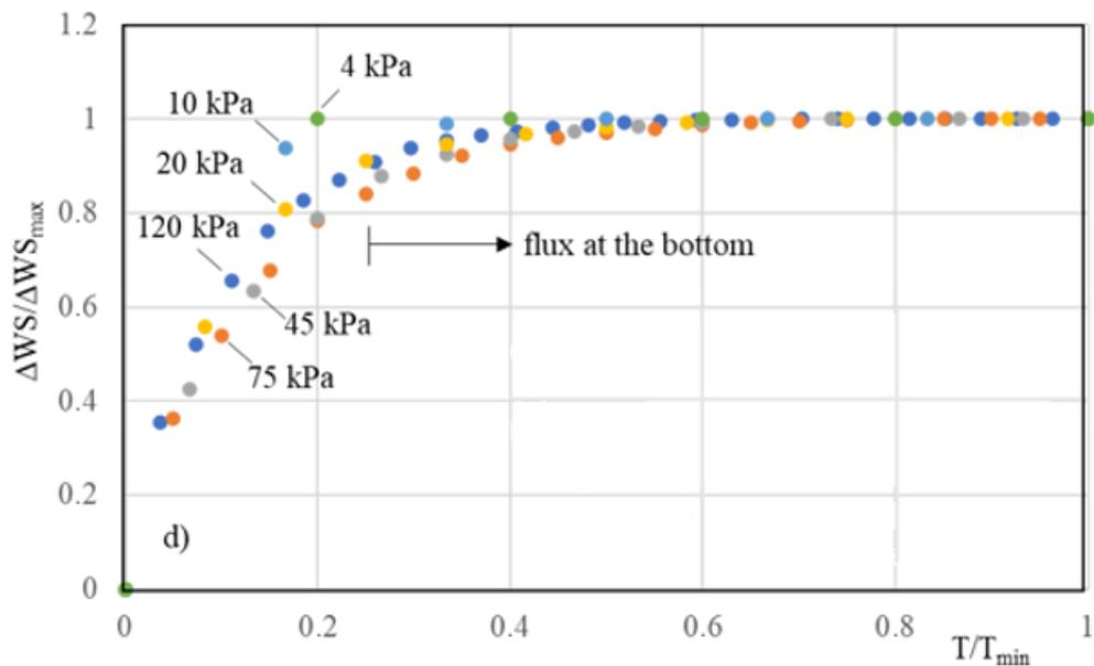
Figure 5-5. Analysis of E group: no-dimensional maximum water storage increase,  $\Delta WS_{max}$ , against no-dimensional minimum time,  $T_{min}$ , to achieve equilibrium.
