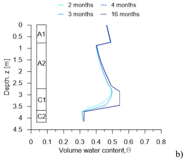
Figure 6-4. Results along the vertical profile of the Pozzano section on 25<sup>th</sup> December 1996 (15 days before the critical event): a) distribution of pore water pressure; b) distribution of volumetric water content.
