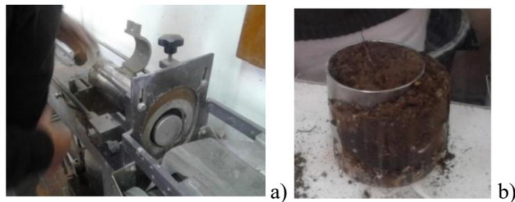
*Figure 3-22. a) Soil specimen extrusion from the undisturbed sample; b) Soil specimen after extrusion (Dias, 2019).*
