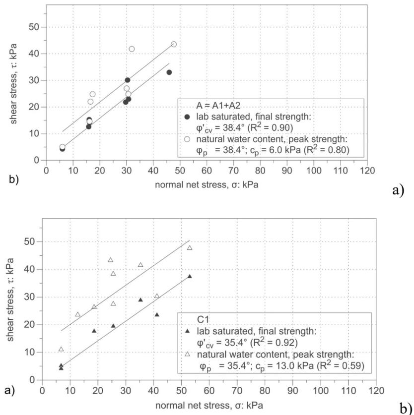
Figure 3-18. Value of shear strength measured in direct shear tests as a function of net normal stress: a) soil C1 and b) soil A1+A2 (Forte et al., 2019).
