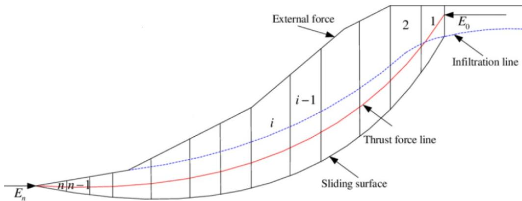
Figure A-5. An example of slope subdivision using the slice method (modified from Huang et al., 2020).
