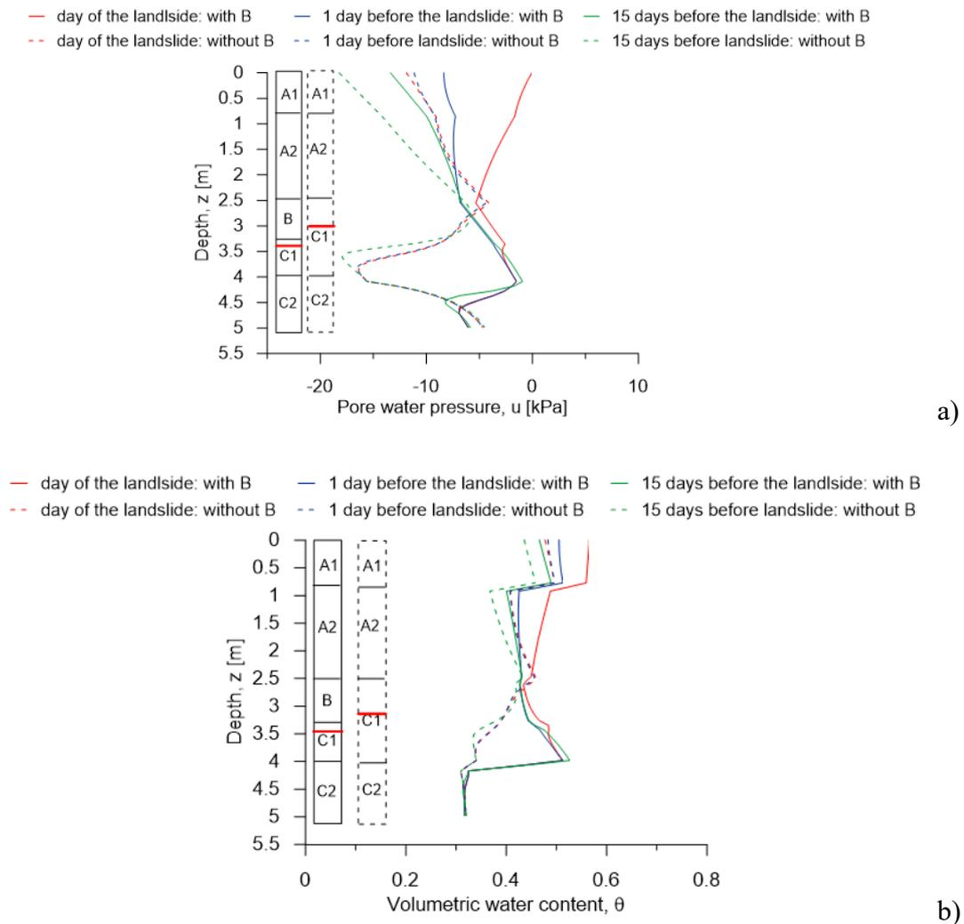
Figure 7-18. Results for Pimonte section in presence of B soil on 10<sup>th</sup> January 1997 and in absence of B on 23<sup>th</sup> November 1996: a) distribution of pore water pressure along the control surface (black dashed line in Figure 7-12) on day chosen, 1 day before and 14 days before; b) distribution of volumetric water content along the control surface on day chosen, 1 day before and 14 days before.
