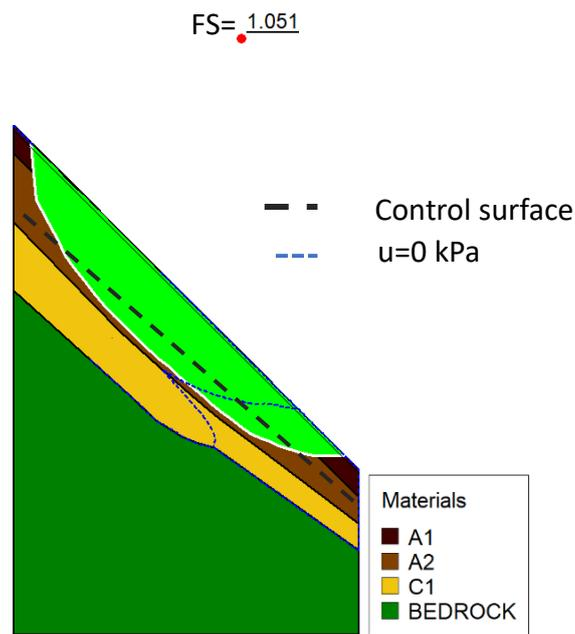
*Figure 7-7. Slope stability analyses for the Pozzano section on 10<sup>th</sup> January 1997: C2 soil replaced by C1 soil*
