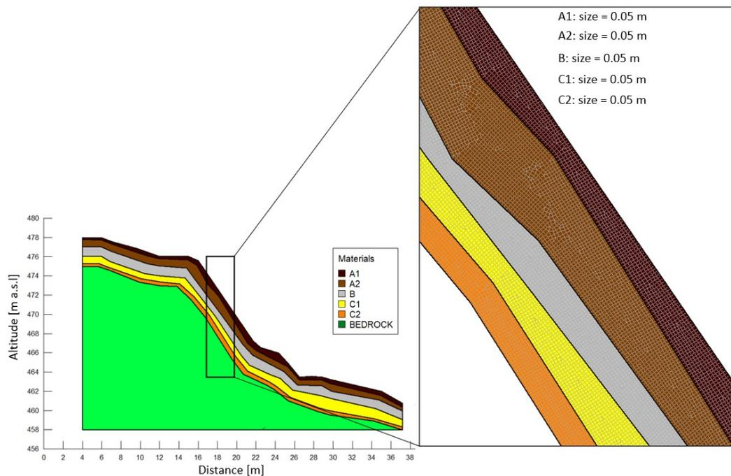
Figure 4-4. Pimonte section crossing the triggering area with details of the mesh size.
