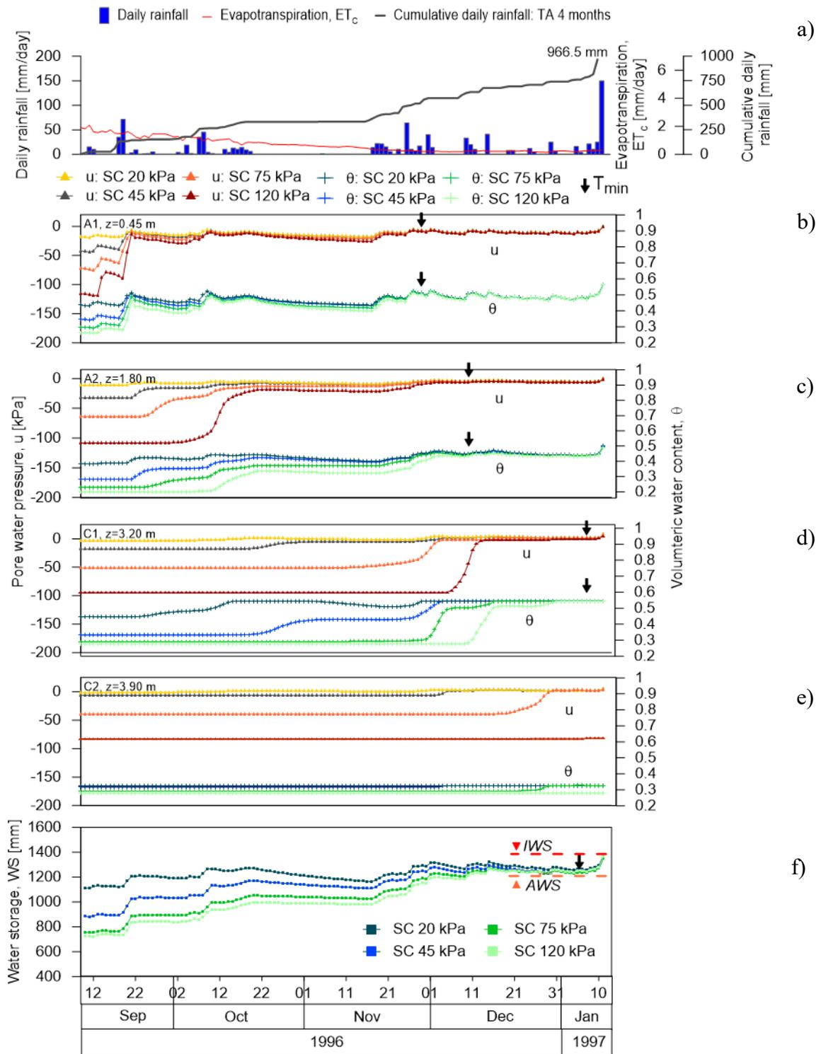
Figure 6-17. Results of analyses of C group for the Pozzano section: a) daily rainfall recorded by the Castellammare di Stabia rain gauge, daily crop evapotranspiration calculated from 10<sup>th</sup> September 1996 to 10<sup>th</sup> January 1997 and cumulative daily rainfall; b) pore water pressure and volumetric water content over time at control point of A1 soil; c) A2 soil; d) C1 soil; e) C2 soil; f) volume of water stored by the slope over time, WS.
