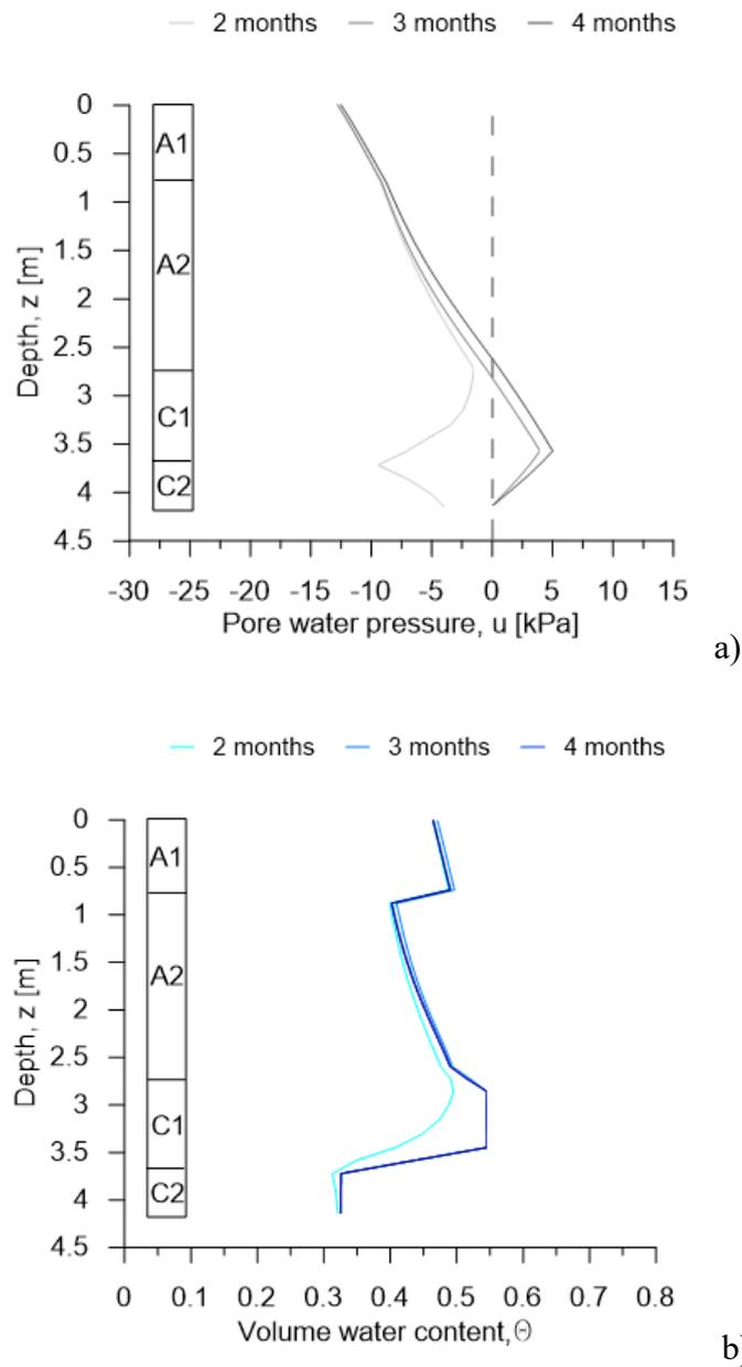
Figure 6-10. Results along the vertical profile of the Pozzano section on 6<sup>th</sup> January 1980 (4 days before the end of the analyses): a) distribution of pore water pressure; b) distribution of volumetric water content.
