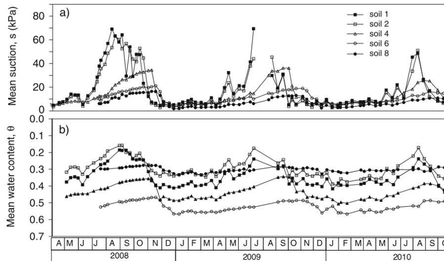
Figure 2-27. Monitoring results: mean suction (a), mean volumetric water content (b) in soil 1, 2, 4, 6 and 8 (Modified from Pirone et al., 2015a)
