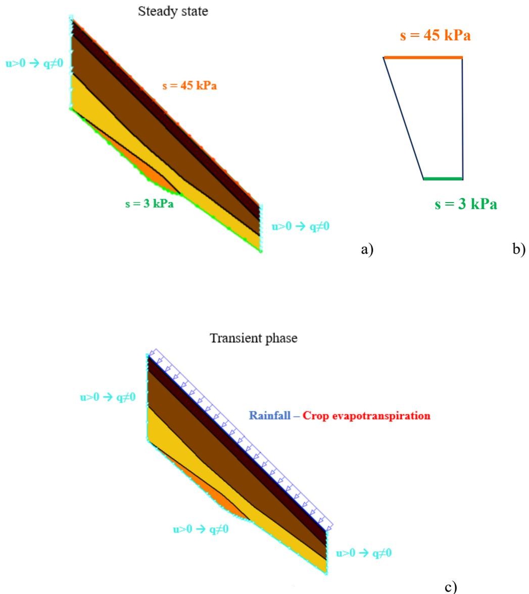
Figure 4-8. An example of hydraulic boundary conditions set for the Pozzano section: a) starting boundary condition; b) starting suction profile; c) hydraulic boundary conditions during the transient phase.
