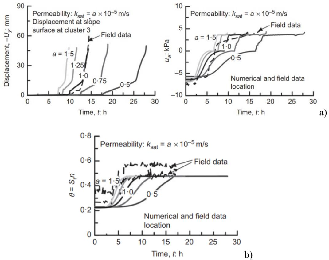
Figure 2-36. The effect of the saturated hydraulic permeability on: a) the evolution of displacements; and pore pressure; b) volumetric water content (Sitarenios et al. 2021).
