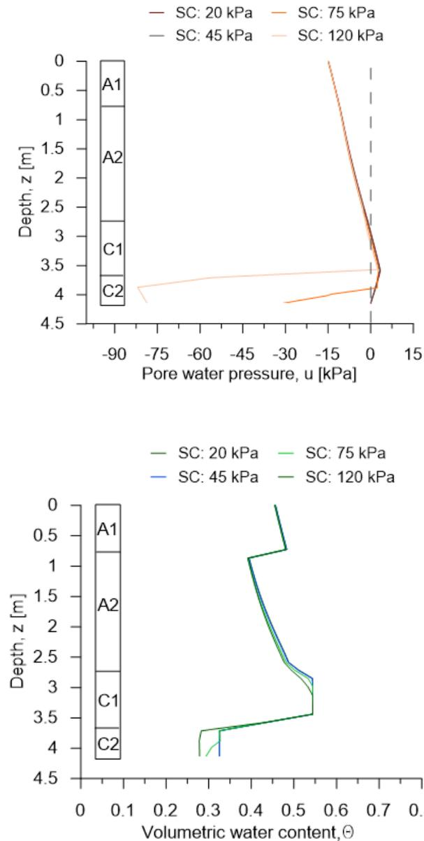
Figure 6-19. Results of analyses of C group along the vertical profile of the Pozzano section on 3<sup>rd</sup> January 1997 (7 days before the landslide): a) distribution of pore water pressure; b) volumetric water content.
