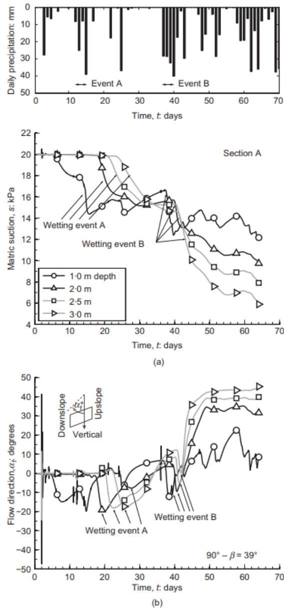
Figure 2-32. Evolution of matric suction at different depths for the main vertical of interest (slope angle  $\beta = 51^\circ$ ) and (b) direction angle of water flow vectors (modified from Laloui et al. 2016).
