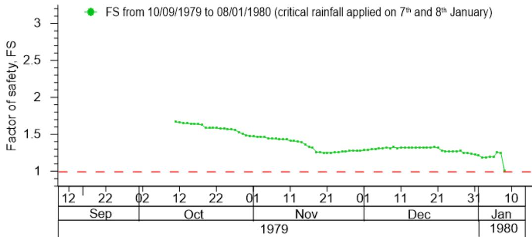
Figure 6-14. Slope stability analysis for Pozzano section: minimum factor of safety, FS, from 10<sup>th</sup> October 1979 to 8<sup>th</sup> January 1980 (critical rainfall of 25 mm and 150 mm on 7<sup>th</sup> and 8<sup>th</sup> January).
