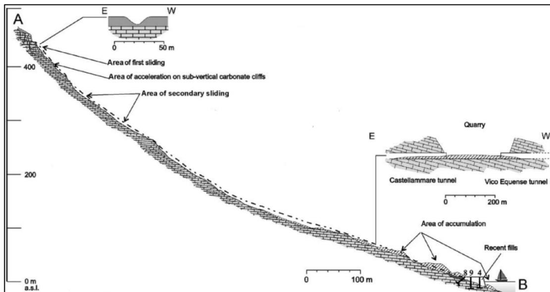
Figure 3-6. Geological section of the Pozzano landslides (modified by Calcaterra and Santo, 2004).
