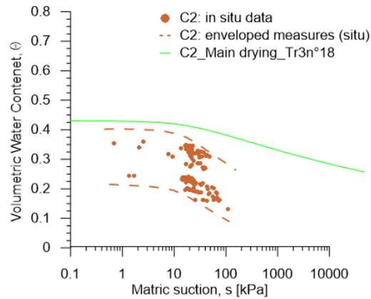
Figure 3-31. C2 soil. Matric suction and volumetric water content from in situ measurements; retention curves from laboratory tests (Dias, 2019); lower envelope of on-site measurements.
