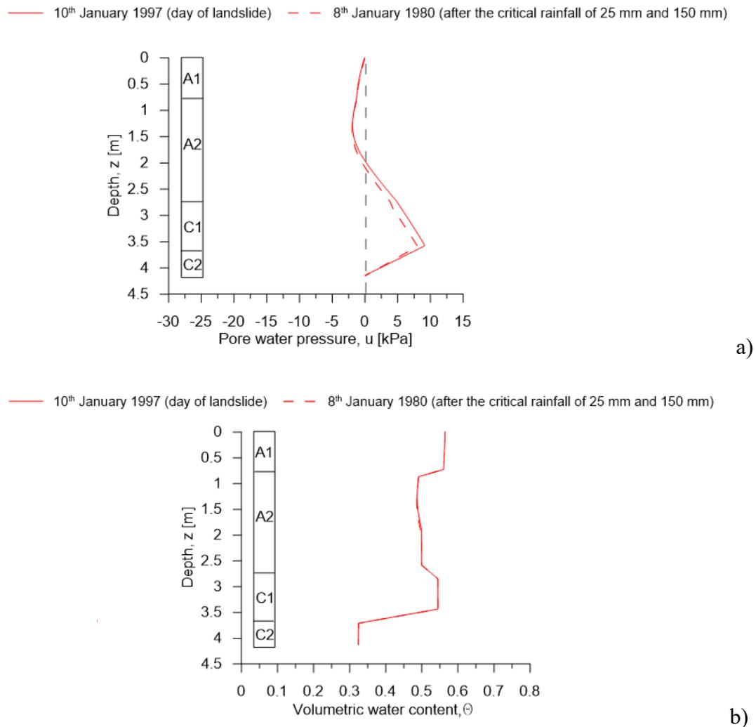
Figure 6-15. Results along the vertical profile of the Pozzano section on 10<sup>th</sup> January 1997 (day of landslide) and on 8<sup>th</sup> January 1980 when the critical rainfall of 25 mm and 150 mm was applied on 7<sup>th</sup> and 8<sup>th</sup> January: a) distribution of pore water pressure; b) volumetric water content.
