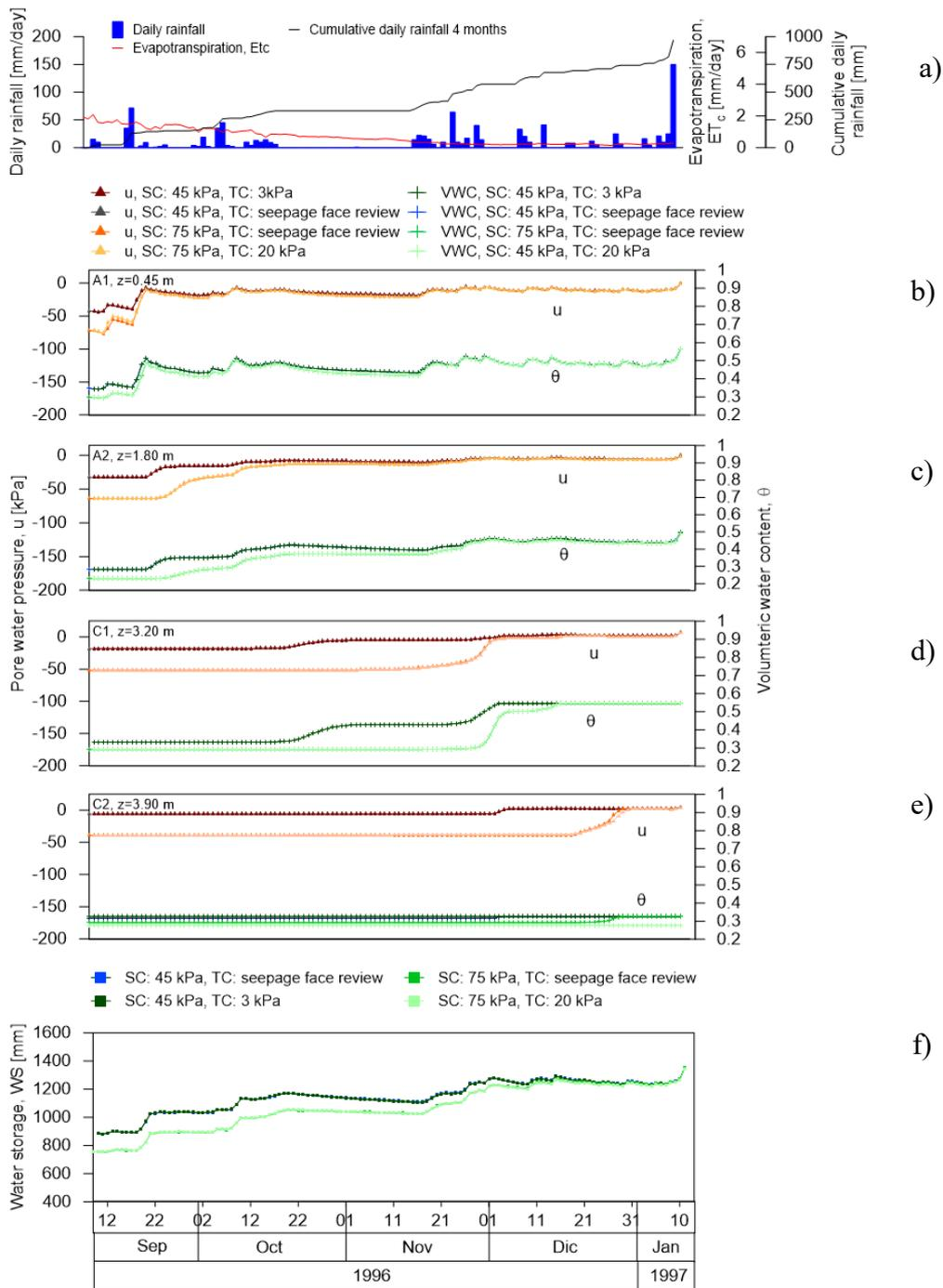
Figure 8-1. Results of analyses of I group for the Pozzano section: a) daily rainfall recorded by the Castellammare di Stabia rain gauge, daily crop evapotranspiration calculated from 10<sup>th</sup> September 1996 to 10<sup>th</sup> January 1997 and cumulative daily rainfall; b) pore water pressure and volumetric water content over time at control point of A1 soil; c) A2 soil; d) C1 soil; e) C2 soil; f) volume of water stored by the slope over time,  $WS$ .
