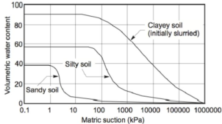
Figure 2-8. Water retention curves of sandy, silty and clayey soils (Fredlund and Xing, 1994).
