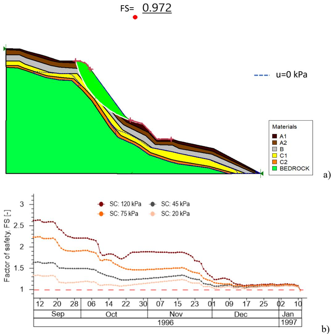
Figure 6-27. Slope stability analyses of D group for the Pimonte section: a) sliding surface relative to the triggering of landslides due to the event occurring on 10<sup>th</sup> January 1997; b) minimum safety factor, FS.
