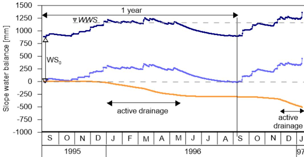
Figure 6-6. Water storage variation, cumulative water drainage and water drainage from bottom edge for Pozzano section from 10<sup>th</sup> September 1995 to 10<sup>th</sup> January 1997.
