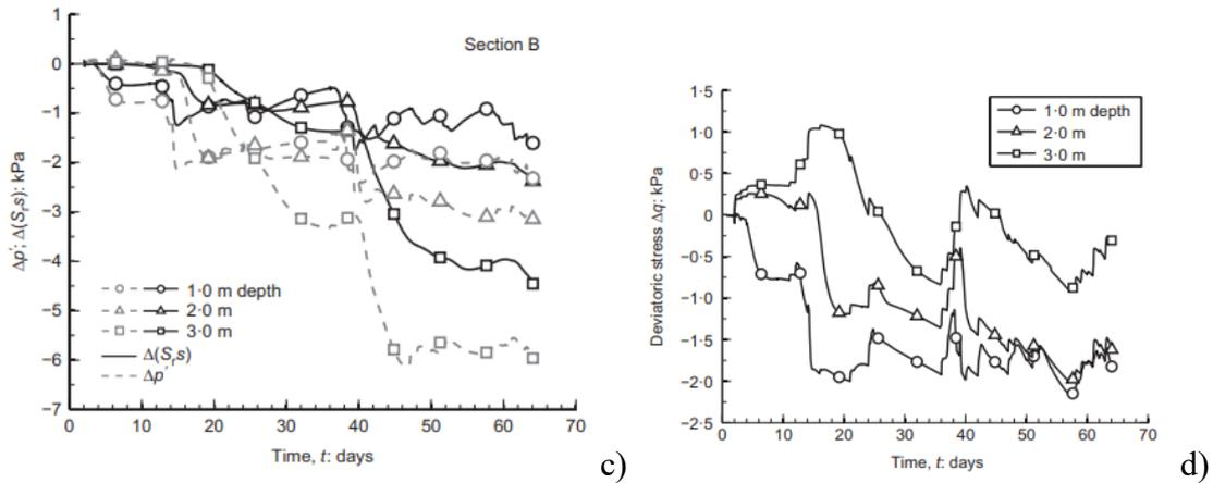
Figure 2-33. Results of analysis: a) evolution of volumetric strains; b) variations deviatoric plastic strains  $\epsilon_p^d$ ; c) variations in mean effective stresses  $\Delta p' = p' - p'_{t=0}$  at 1, 2 and 3 m of soil depth; d) deviatoric stresses  $\Delta q$  at 1, 2 and 3 m soil depth (modified from Laloui et al. 2016).
