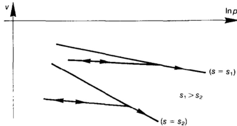
Figure 2-12. Proposed variation of specific volume with net mean stress and suction along virgin and unloading-reloading paths (Alonso et al. 1990)
