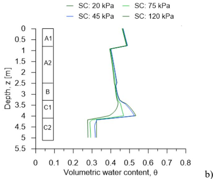
Figure 6-26. Results of analyses of D group along the vertical profile of the Pimonte section on 27<sup>th</sup> December 1996 (14 days before the critical event): a) distribution of pore water pressure; b) volumetric water content.
