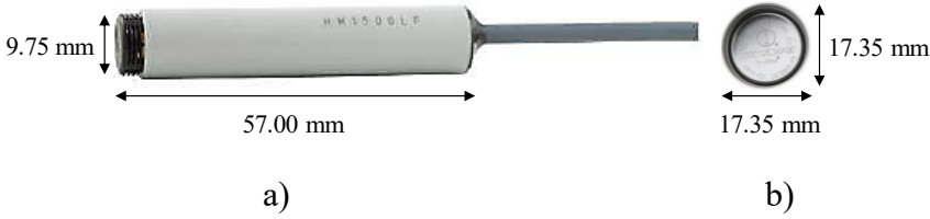
Figure 3.8 Relative humidity measurement instruments: a) hygrometer HM1500LF; b) i-Button
