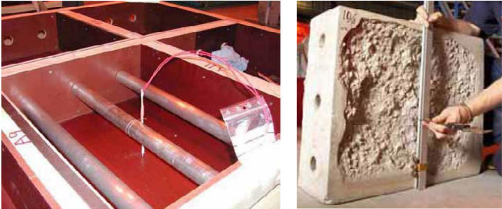
*Figure 31: Image of sampling casings with sheaths for post-tension cables and thermocouples; b) Image of the specimen after the test (by [45]).*
