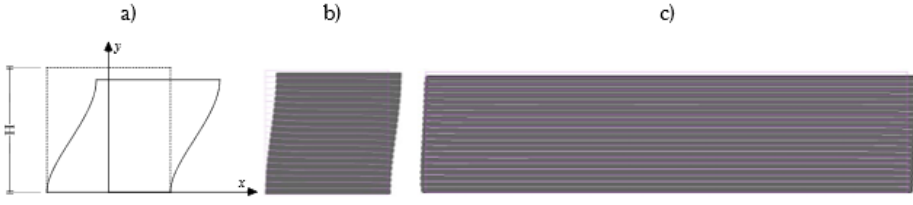
Figure 5.4: Deformed bearing configuration at buckling load: a) adapted from Tsai [33], b) t_e = 2 mm, G_e = 0.4 MPa, S_2 = 1 , b) t_e = 2 mm, G_e = 0.4 MPa, S_2 = 4 .
