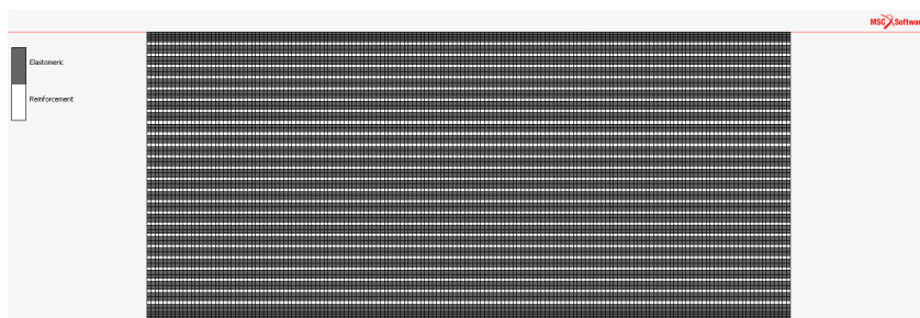
Figure 3.4: Geometry and discretization of a FREI for 2D FEAs in MSC.Marc.
