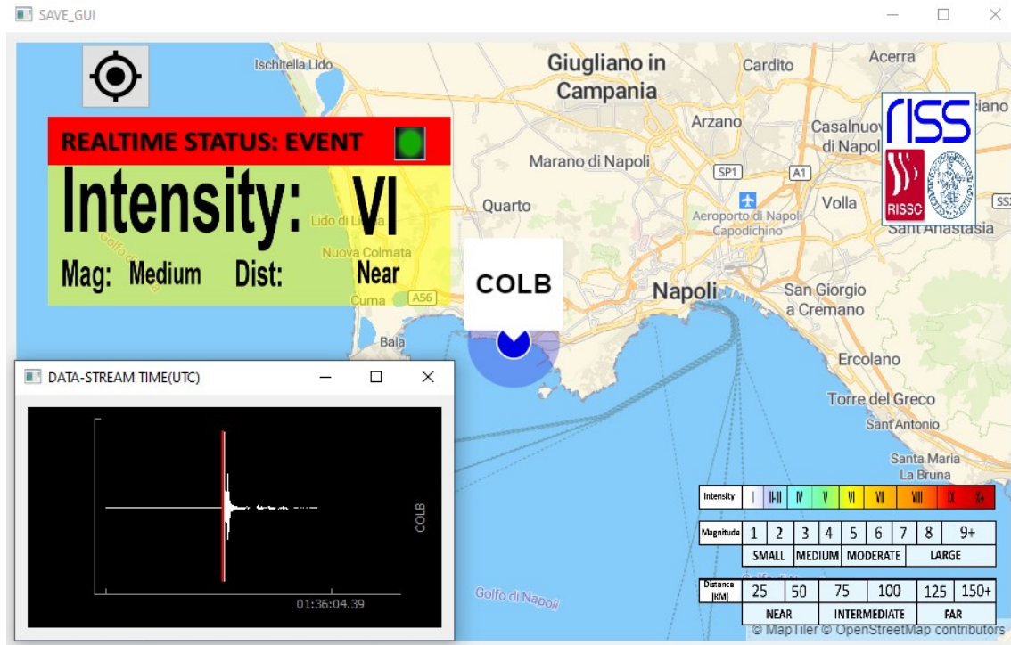
Figure 3.4.6: SAVE graphical interface for the station COLB located at 900 meters from the event epicenter. At this station, the alert is issued for expected event of MMI=6, medium magnitude, nearby the site. The pulsing blue point on the map is the station location. In the bottom right the reference for intensity, magnitude and distance scales are represented. In bottom left the data stream of the signal is shown with the P-wave automatic pick marked with the vertical red line.
