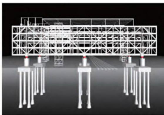
Main Building of Shimizu Corporation , Japan (2003): (80 x 20) m<sup>2</sup> for 6 levels – no. 6 LDRBs (diameter: 1000-1100 mm)
